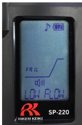
Fault alarm display example: Low flow rate
